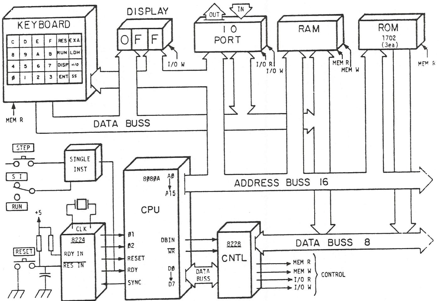
Figure 1. Operational block diagram of MST-80B Microcomputer trainer.
