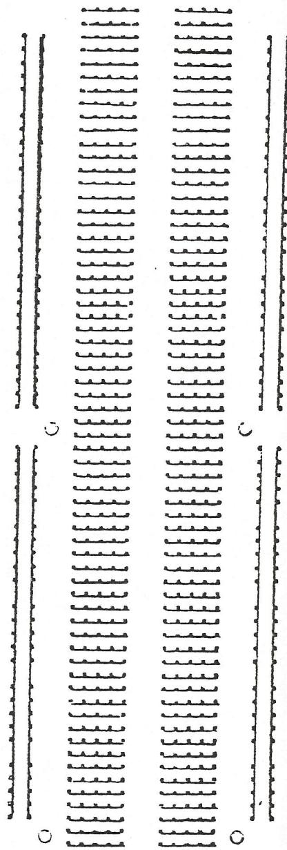
Figure 5 Breadboard Hidden Connections
